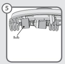
Install a light bulb in each socket.
